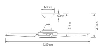
Note: Do NOT install on a raked or sloped ceiling without the use of the optional 38° Ceiling Kit, as this will damage the receiver housed in the canopy.
